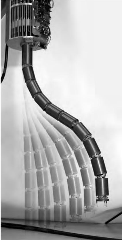
**A composite photo of OC Robotics' Explorer snake robot reveals its flexibility, an asset when the device operates in cramped quarters. (Photo Courtesy OC Robotics.)**
