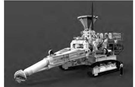
**The collecting machine ROV will pump material in slurry form to the ship.**
