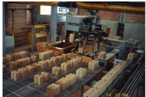
*Figure 3\*: Robotic cutting and sequencing of bricks*
