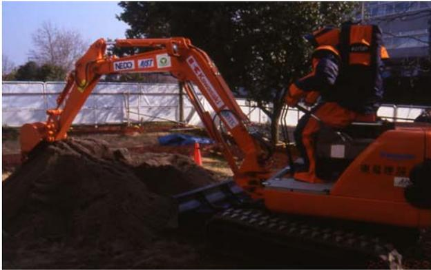
*Figure 17\* shows a humanoid robot riding an excavator*
