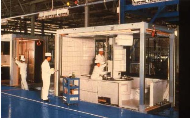
*Figure 7\*: Quality End Control of a box unit with bath room from a flexible manufacturing system*
