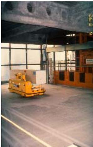
Figure 13\*: Construction material distribution robot
