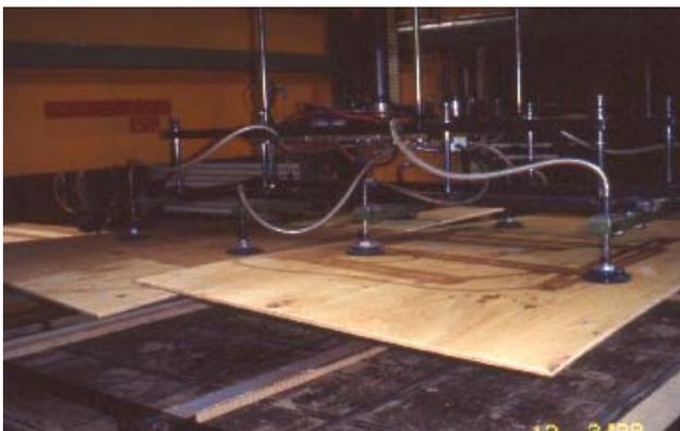
*Figure 5\*: Robotic vacuum gripper for customized wooden panel production*
