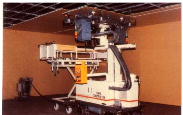
Figure 12\*: An interior finishing robot for mounting of suspended ceilings
