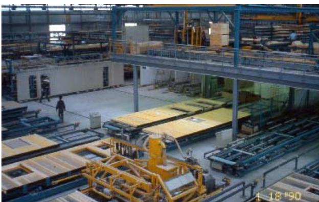
*Figure 6\*: overview of a factory with robotic nailing and gluing bridges for wooden panel production.*
