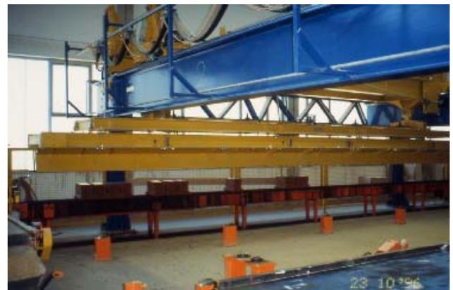
*Figure 4\*: Robotic spacing and positioning of bricks for customized masonry wall prefabrication*
