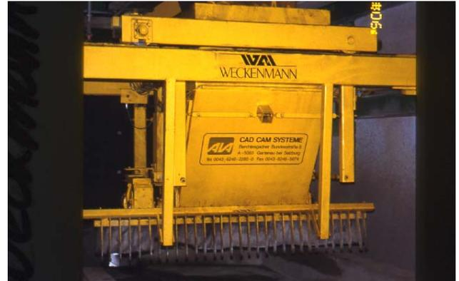
*Figure 2\*: Robotic Concrete distributor*
