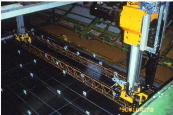
*Figure 1\*: Flexible CAD/CAM gantry type production unit for PC floor, wall and roof elements using two robotic endeffectors for reinforcement positioning*
