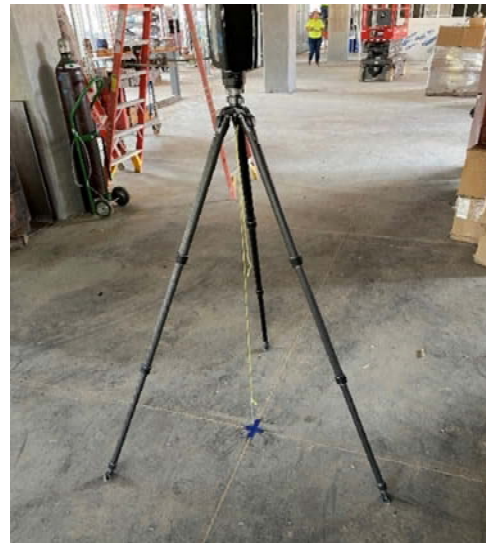
Figure 1: Example terrestrial LiDAR scanning (TLS) approach using a tripod.
