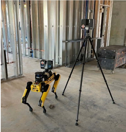
Figure 4: Hardware setup of tripod based scanner and robot based scanner.
