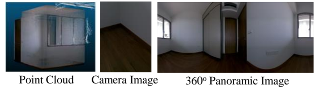
Figure 2. Data captured by scanner on the robot.
