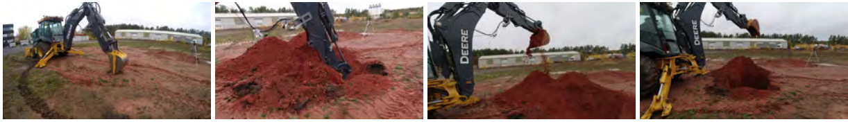
Figure 2. Image of the start of the four different digging phases of the excavation process, from left to right: "Digging", "Move to Dumping", "Dumping", "Move to Digging"
