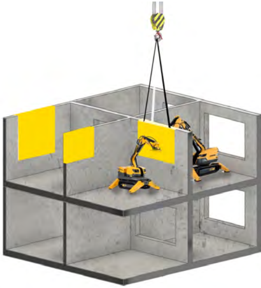
Figure 5. Conceptual visualization of the planned usecase: Top-down deconstruction approach with tower crane
