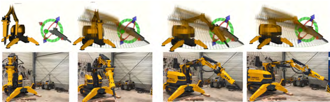
Figure 4. Snapshots of the BROKK 170 tracking a trajectory in the TCP-level. The grey tool can be interactively positioned and rotated by the operator defining the desired tool pose. According to the desired tool pose, a TCP trajectory and the corresponding joint trajectories (upper row) are generated. The joint trajectories' joint angle changes are then converted into the PWM signals to move each actuator along the desired joint trajectory (lower row).
