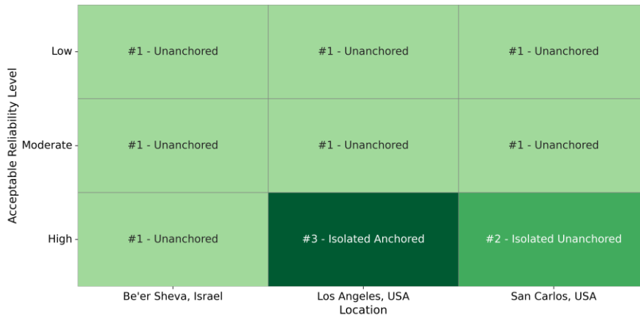
Figure 7 - Optimal generator configuration across various locations and acceptable reliability levels. Each cell represents the most cost-effective diesel generator type that satisfies the target reliability at the specified site
