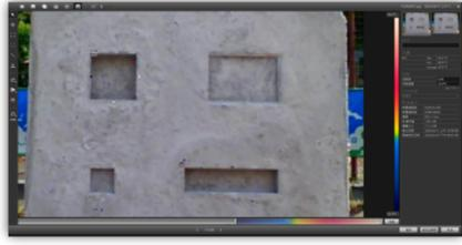
Figure 3. Example of selecting defect temperature value in the visible light image
