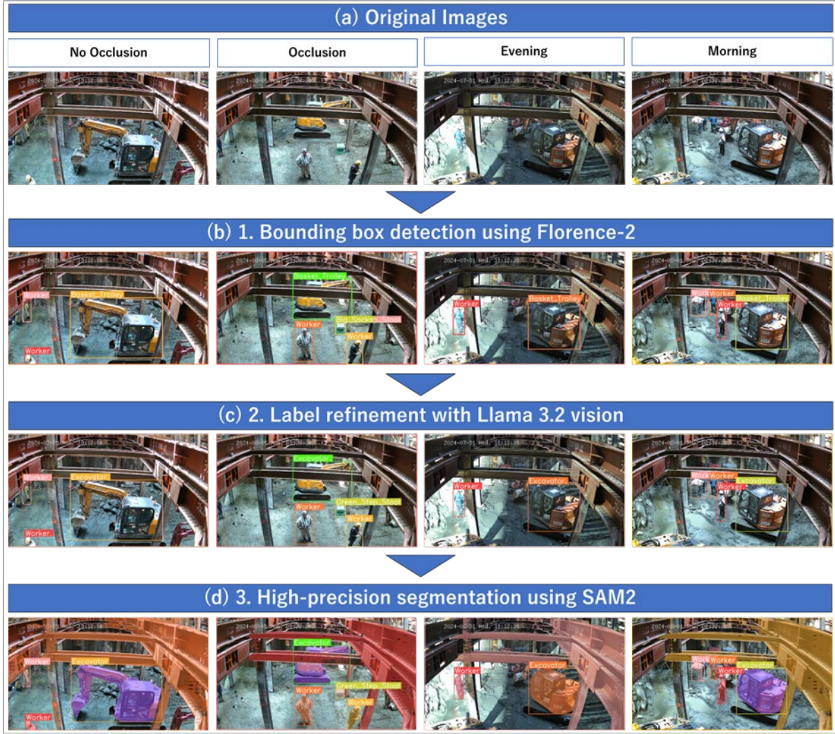
Fig. 5. Results of bounding box estimation (Florence-2), label prediction (Llama 3.2-Vision), and segmentation (SAM2).
