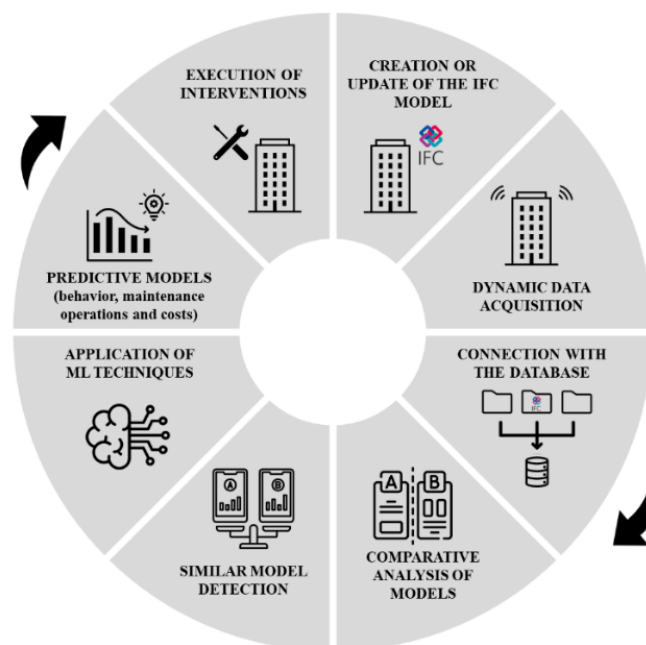
Fig. 1. Schematic of the proposed cyclical process for predictive maintenance.
