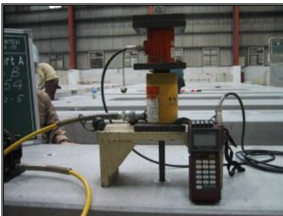
Figure 10. Pulling test on insert plug A and C
