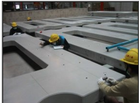
Figure 7. Products check of slab tracks
