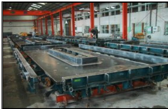
Figure 4. Molds for slab tracks
