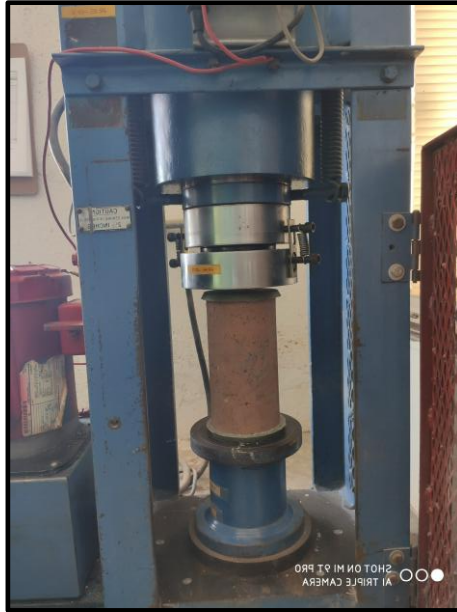
Fig. 3. Compressive strength test
