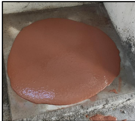
Fig. 2. Slum Flow test
