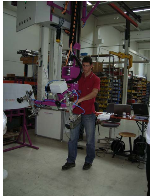
Fig.4. COBOT operated in manual mode
