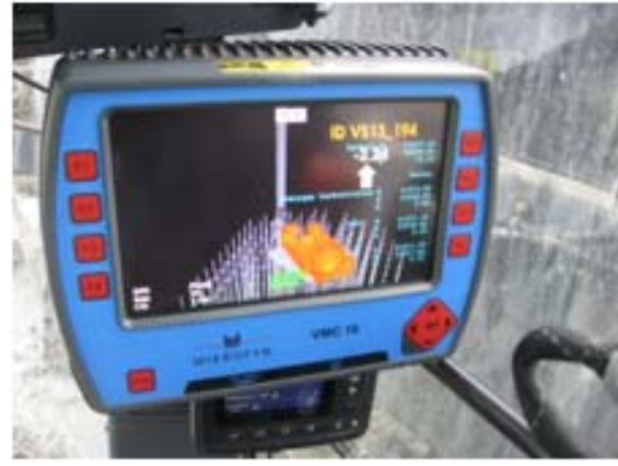
Fig.8. An user-interface of the 3-D control system for deep stabilization machine.
