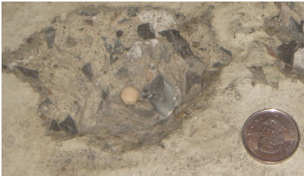
Fig.2. Use of Artificial Target for Scale Calibration
