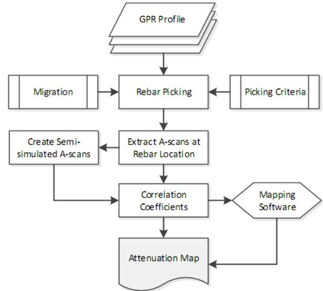
Figure 3. Procedure for mapping attenuation of bridge deck
