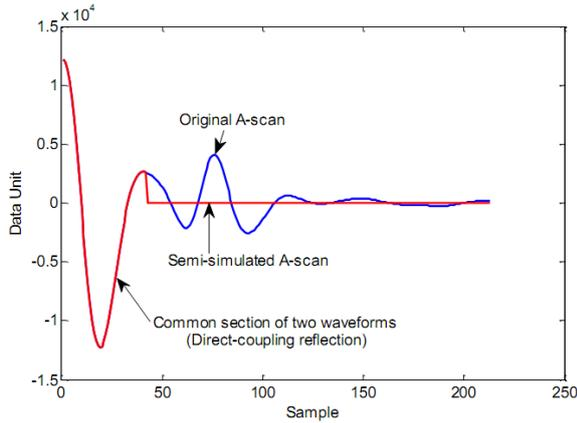
Figure 2. Comparison between original and semi-simulated waveform
