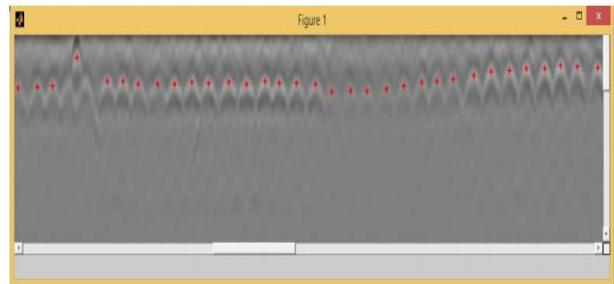
Figure 4. Example performance of rebar picking algorithm
