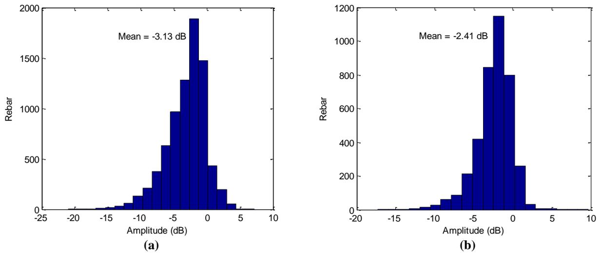
Figure 9. Histogram of depth-corrected amplitude for (a) Haymarket bridge deck and (b) Pohatcong bridge deck.
