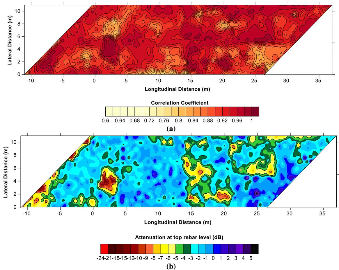
Figure 7. GPR attenuation maps for Pohatcong bridge deck with (a) Proposed method and (b) ASTM standard
