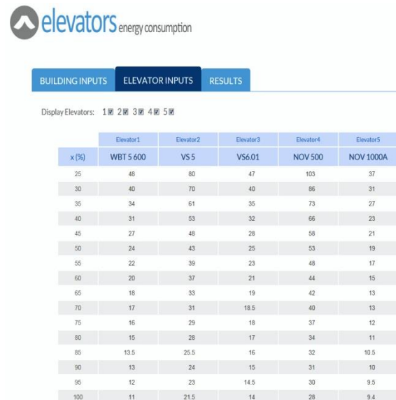
Figure 7. Elevator inputs - values of E_c [Wh/tm]
