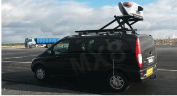
Fig. 4. Trimble MX8 mobile mapping vehicle (Geotrim Oy)
