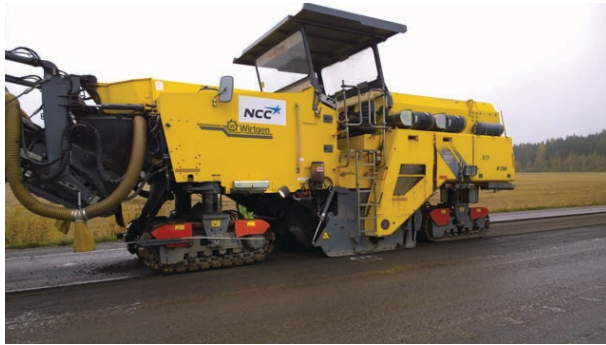
Figure 10. NCC Roads Oy, Milling machine own 2-D automatic (Finnmap Infra Oy).
