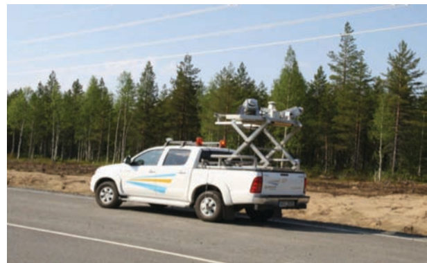
Fig. 3. GEOVAP, spol. s r. o. mobile mapping (LYNX Mobile Mapper) vehicle (Geovap).
