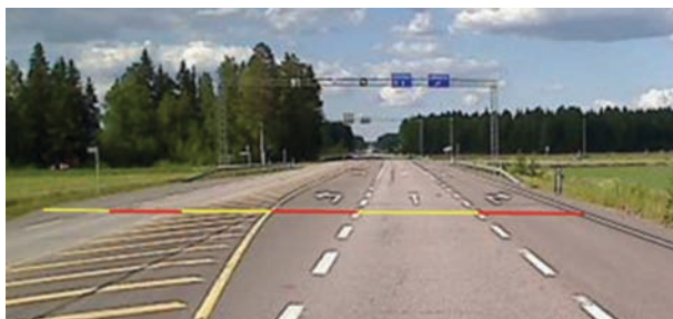
Fig. 5. Placing of 3-D break lines in Vt6 (Roadscanners Oy).
