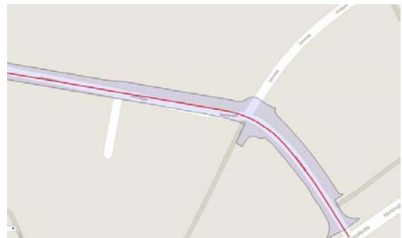
Fig. 4. Cutting surface design added in the collaboration cloud. Also showing road centreline (red line).
