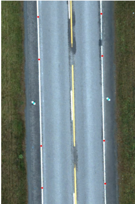
Figure 5. Layout of the reference points (red) and signal paint patterns (white with blue dot).
