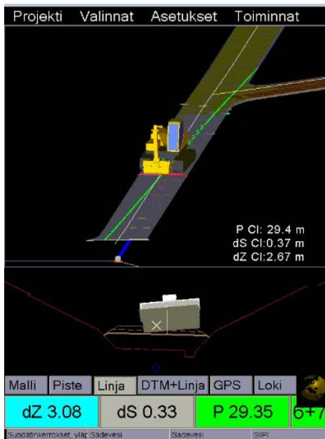
Figure 1. Picture of a Novatron 3D excavator's interface.
