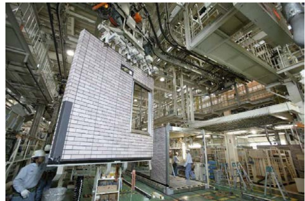
Figure 5. The concept of Robotic Industrialization applied by the company Sekisui Heim to industrially personalize buildings on the assembly line (Image: courtesy of Sekisui Heim).
