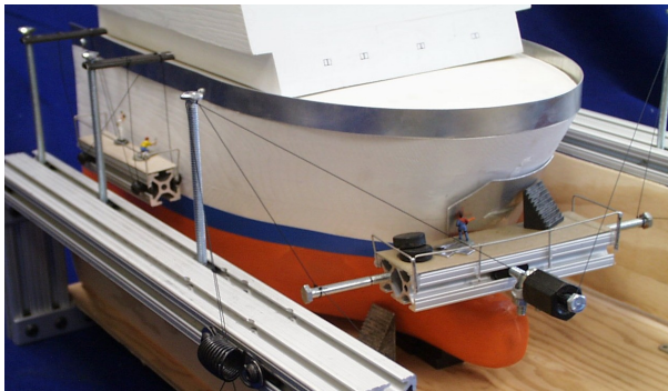
Figure 1. NIST Flying Carpet 1:120 scale concept model showing the ship bow/stern access configuration (right) and the ship side access configuration (left).
