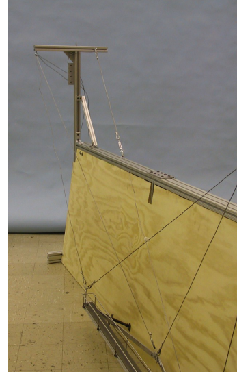
Figure 4. Photograph of the Flying Carpet 1:12 scale model shown in the ship side access configuration. The 1:12 scale model shows a tower attached to the dry dock wing wall and the platform pushing against the wall.
