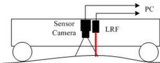
Figure 12. Device with LRF
