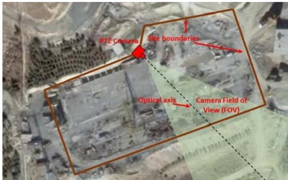
Figure 1. Mapping the camera in the site plan
