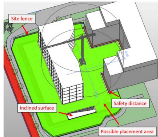
Figure 2. Interactive rule checking: possible placement area of a tower crane
