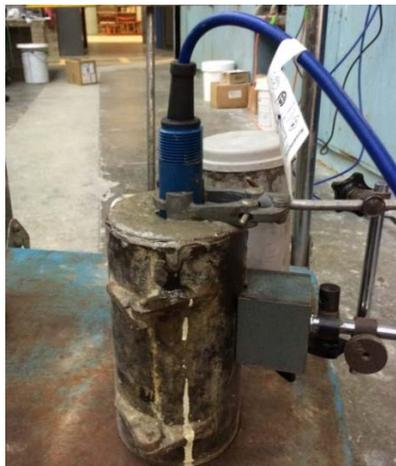
Figure 2. set-up of pH sensor embedment
