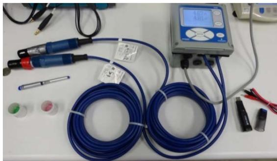
Figure 1. Experiment setup of the pH Sensor System (Emerson Ptd.)
