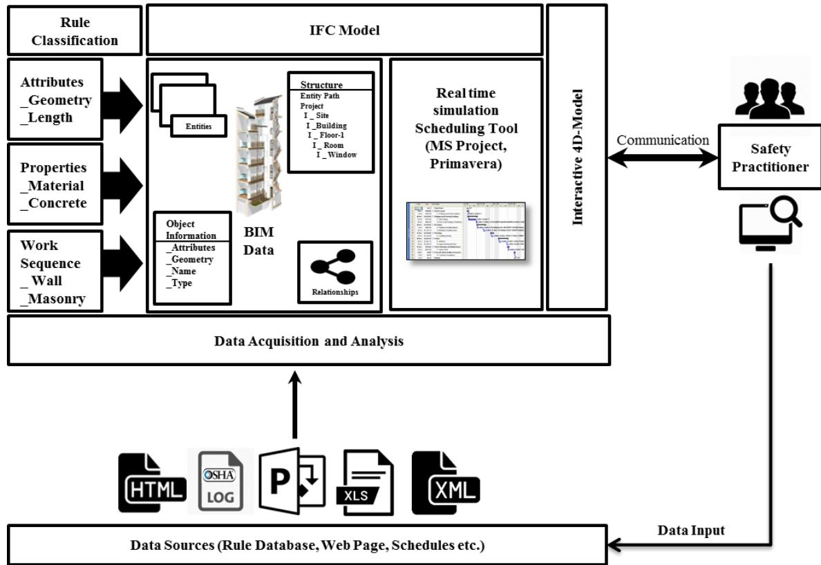
Figure 1. System Framework for applying safety rules with BIM model
