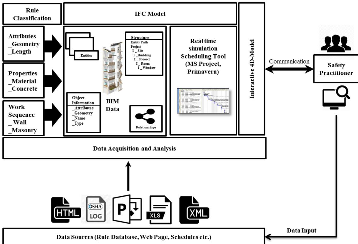
Figure 1. System Framework for applying safety rules with BIM model
