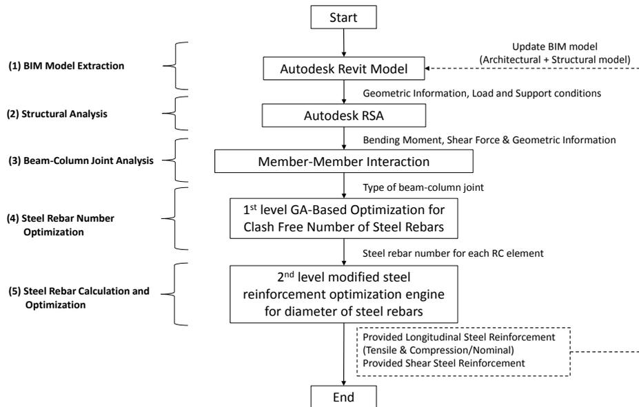
Figure 9. BIM-based automated clash free steel rebar design optimization framework tool
