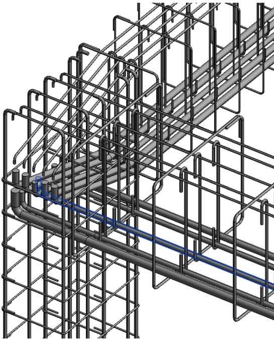
Figure 11. 3D output of one of the beam-column joints of the considered RC frame
