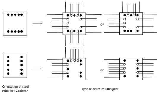
Figure 6. Assignment of steel rebar in RC elements depending on the orientation of RC column reinforcement and type of beam-column joint
