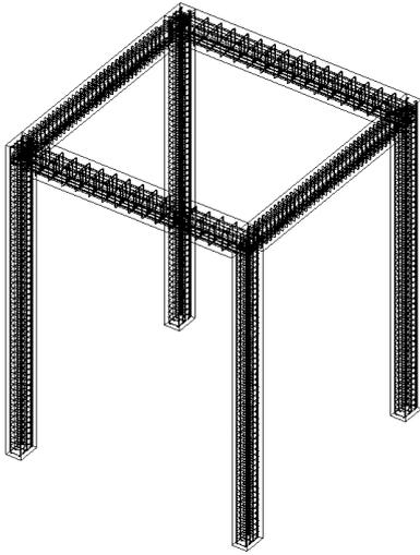
Figure 10. Automated 3D view of the optimized steel rebar for the considered RC frame
