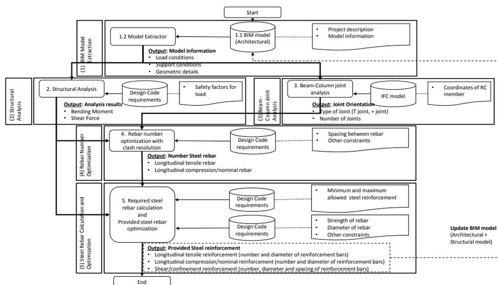
Figure 1. The proposed BIM-based automated clash free steel rebar design framework
