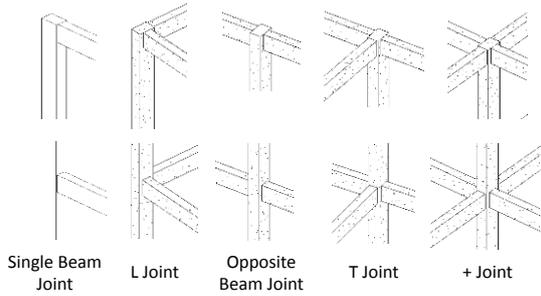
Figure 2. Various types of beam-column joints generally encountered in an RC frame
