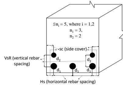
Figure 3. Horizontal and vertical rebar spacing for an RC member
