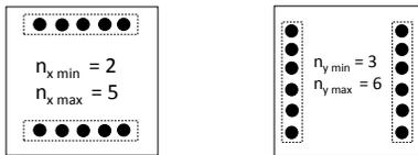
Figure 5. Steel rebar range in x any y directions for an RC column
