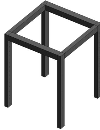
Figure 8. A one-storey fixed end RC frame
