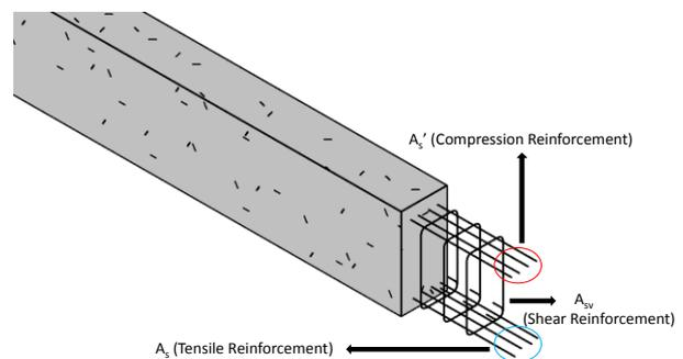
Figure 7. Steel reinforcement optimized by hybrid GA-based steel reinforcement optimization engine for a given RC beam
