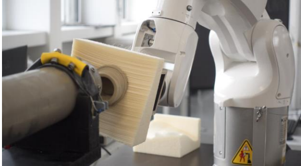
Figure 9. Robotic system Demonstrating additive and subtractive fabrication.
