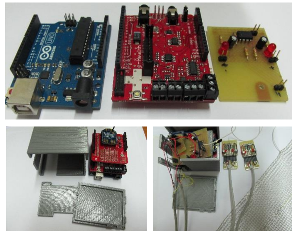
Figure 3. Hardware of the capacitive ECG, Arduino, e-Health shield & Driven-Ground-Plane board (top), case & assembled boards (bottom left), assembled ECG module including electrodes (bottom right).
