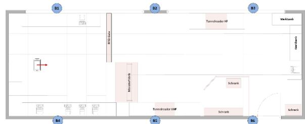
Figure 2. Floor plan of the test laboratory. Blue circles indicate the position of BLE beacons. Red spaces show objects with heights over 1.5 m.
