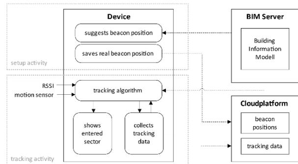
Figure 8. Proposed system architecture for the sector location tracking algorithm
