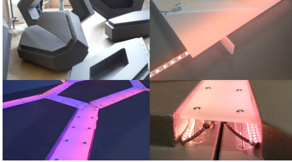
Figure 4: Top: Single protoCELLs (Left); testing Perspex ® over LED1 (Right). Bottom: Generated color gradient (Left); Acrylic connections & two LED-strips within the seam of two protoCELLs (Right).
