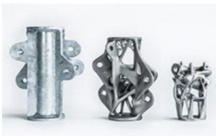
Figure 3. Arup's Optimized Node [29]
