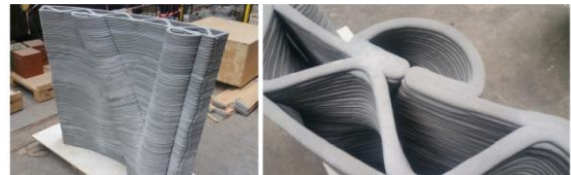
Figure 5. Multifunctional wall element [10]
