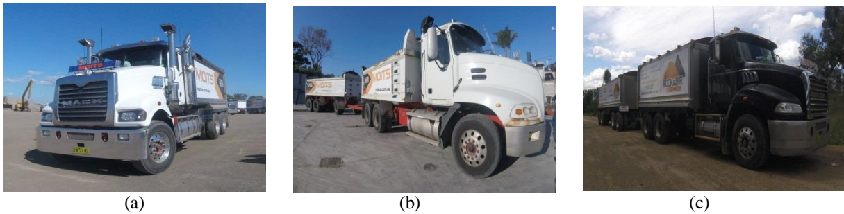
Figure 6. Samples photos of on-road HDVs experimented, (a) a three-axle vehicle without trailer, (b) six-axle vehicle with a trailer, and (c) seven-axle truck with a trailer
