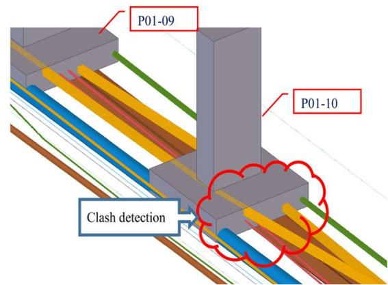
Figure 3. Overlap between pier foundations and pipeline systems
