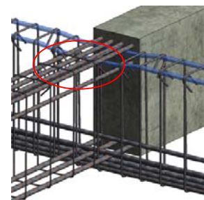
Figure 3. A diagrammatic sketch of beam and girder construction by Revit
