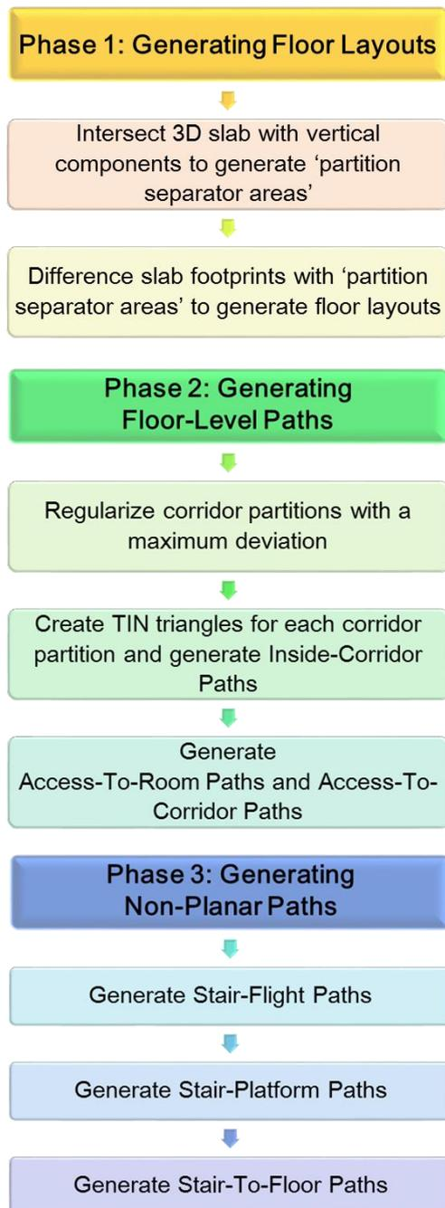
Figure 5. The workflow of generating indoor space topology based on 3D GIS technologies
