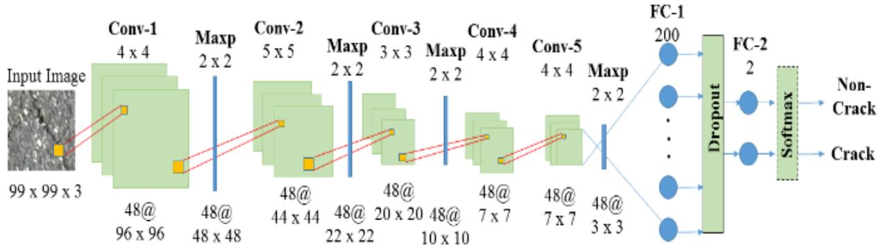
Figure 3: The structure of the Convolutional Network architecture used
