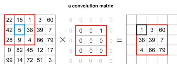
Figure 1: Convolutional operation
