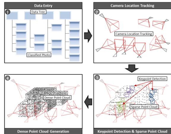
Figure 1. .Input 2D image, Calculation of camera pose, Generation of 3D point-cloud
