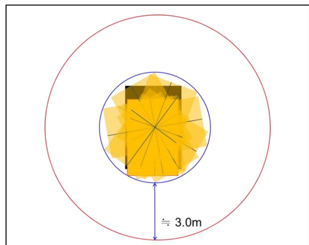
Figure 1. Example of the body rotation of the excavator from a top view
