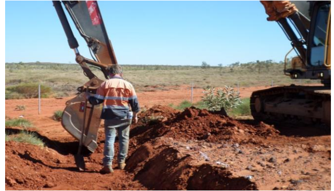
Figure 8. Operator Assisted, Laser Receiver mounted on Shovel
