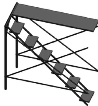
Figure 9. Self-made scaffolding BIM element
