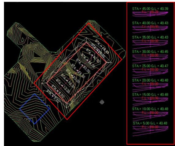
Figure 7. Pad design with station information
