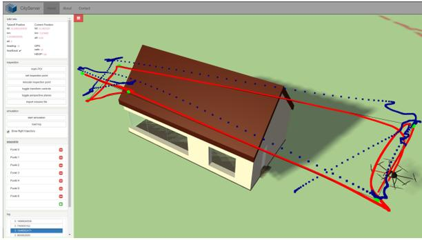
Figure 7: The recorded flight trajectories of the simulation (red) and the field test (blue)
