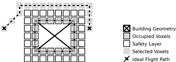
Figure 3: Schematic top-down view of the navigation mesh around a building
