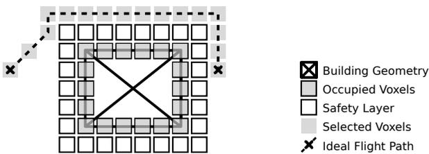
Figure 3: Schematic top-down view of the navigation mesh around a building
