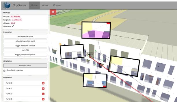
Figure 2: After selecting an element the user is presented with previews of the images the inspection will yield
