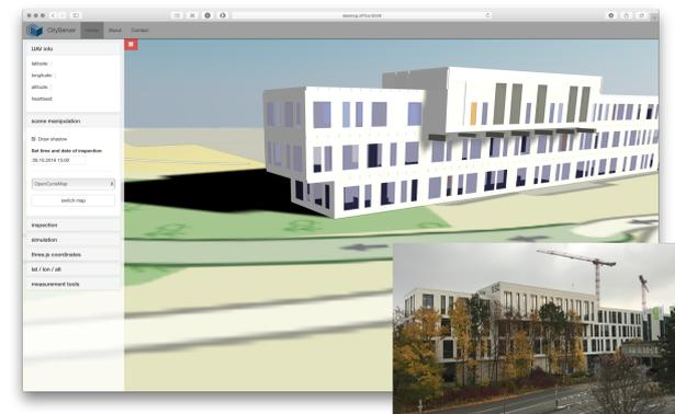
(a) The BIM loaded in the inspection planner application and the real building
