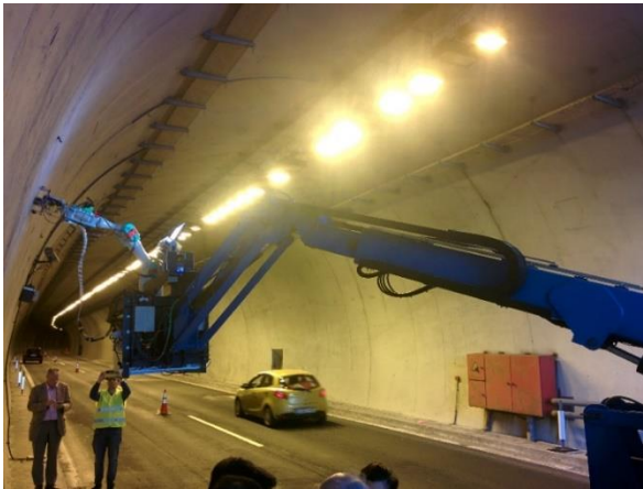
Figure 1. ROBO-SPECT is an FP7 European project to design a fully autonomous tunnel inspection robotic system.
