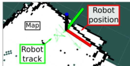
Figure 7: Shows the result of hector\_slam with the robot position and path marked by in the figure. Localisation and mapping errors occur in this example because the RPLIDAR is tilted out of its original plan without any update e.g., using data from an IMU.
