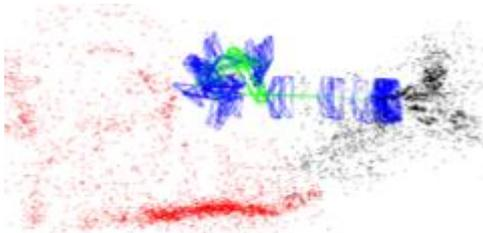
Figure 4: The map produced by ORB-SLAM. The key frame locations can be seen by the blue rectangles, the current keyframe as a green rectangle and the progression of the robot also in green. The red map points show the local visible map.
