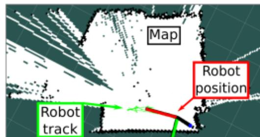
Figure 8: The SLAM result for one set of LIDAR data using Hector SLAM. The robot position, trajectory and map boundaries are shown. Maximum sensor values are also returned in some instances – shown by lines that go outside the map.
