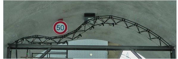
Fig. 12 Shape control of guide frame in model tunnel
