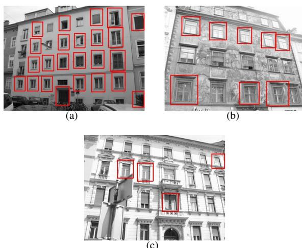
Figure 6. Detections on different facade types and viewpoints. (a) Good detection rate on simple facades with common windows. (b) Decreased performance on complex facade appearance. (c) Despite simple facade few detections due to viewpoint.
