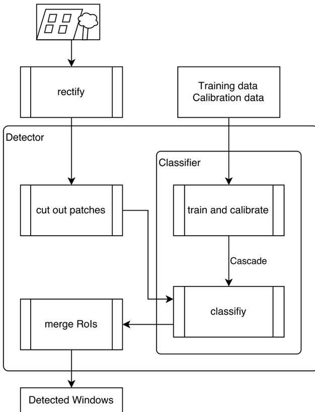
Figure 3. Concept of the proposed detection system. Images are rectified and passed to the detector. The detector cuts out image patches which are classified by a trained and calibrated cascade. Overlapping regions of interest (ROIs) of positive classifications are merged. Resulting ROIs are returned as detected windows.
