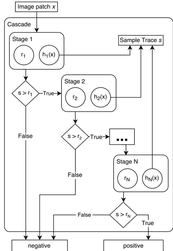
Figure 5. Schematic illustration of the cascaded classification procedure. The weak classifiers of each stage are only evaluated if the sample trace  $s$  is higher than the rejection threshold  $r_i$  of the preceding stage. A sample is positively classified if it passes through the whole cascade. Otherwise it is prematurely declined and negatively classified.
