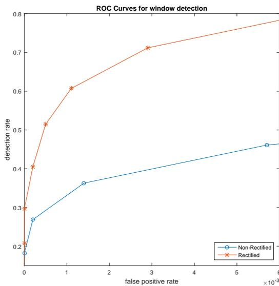
Figure 7. Comparative detection performances of the non-rectified and the rectified classifier by means of their ROC curves.
