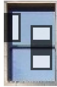
Figure 4. Two Haar-like features at different positions in the image patch, each corresponding to a weak classifier.
